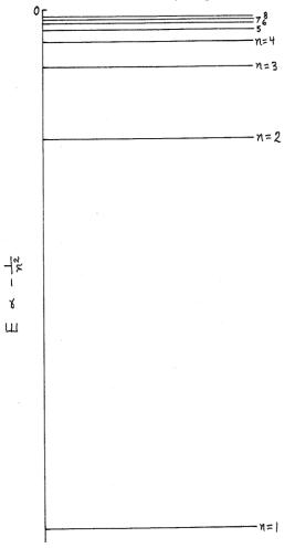
In the ground state, hydrogen's one electron is in the n=1 energy level. There are an infinite number of excited states, where the electron can be in the n=2 energy level or n=3 energy level or any higher level.
